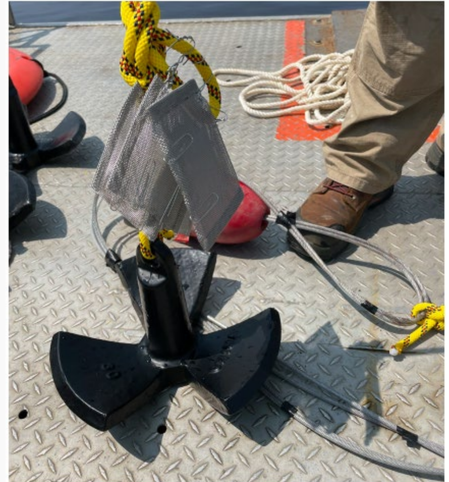
Anchor and buoy assembly for low-density polyethylene deployment
